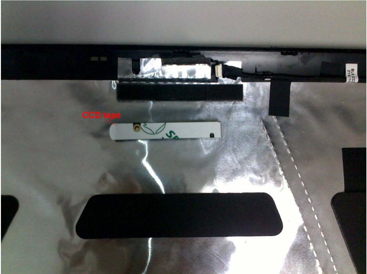
Figure 4-20-3 Camera Module before installing
